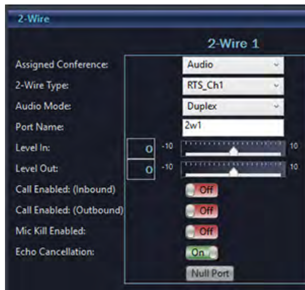
Figure 77 Expanded CU 2-Wire Port Panel
